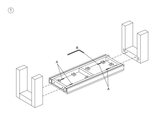
FIX THE LEGS WITH THE TOP USING A SCREWS
