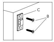
Mark and drill holes for sciews, installing one anti-tip bracket onto the back of your furniture piece in a vertical position.
