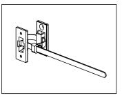
Ensure your furniture is moved into its final position and pull the strap threaded through both anti-tip brackets, until it is parallel with the wall.
