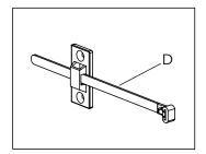
Thread the strap through both anti-tip brackets mounted onto the wall and your furniture.
