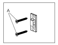
Mark and drill holes for scews before installing another bracket onto the wall, taking care to line it up with the mounted furnitue bracket.
