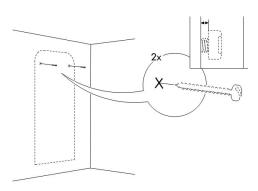
(3.) Place the hangers at the back of the mirror over the screws.
